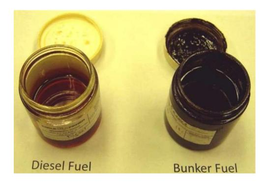
During the combustion of bunker fuel (propulsion of marine vessels) the impurities cause several environmental issues, mainly air pollution (greenhouse gas emissions) and carbon black particle emissions.
